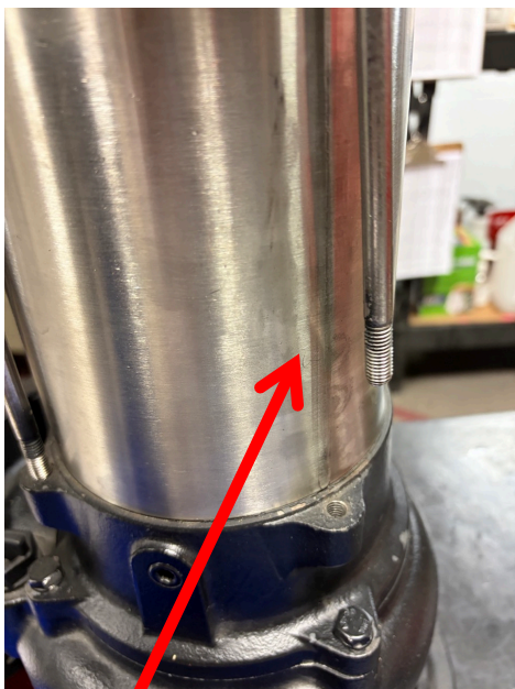
Align all bolts with the weld seam.
